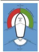
All vessels must have navigation lights in accordance with the International and Inland Navigation Rules. Many towing vessels are found to have inoperable stern, masthead, and sidelights. In some instances the installation of these lights was found to conflict with the International
